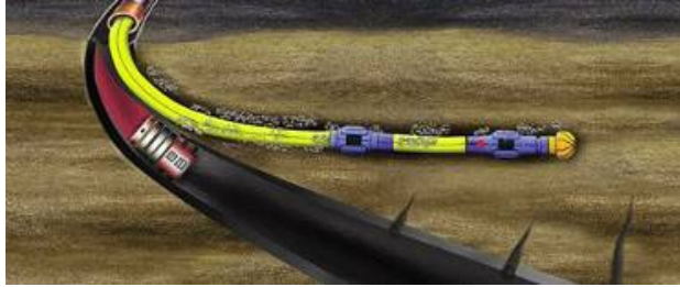
Figure 2-14 Through Tubing Drilling (Photo: Statoil)
